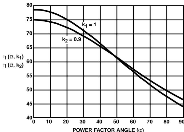
FIGURE 1. IDEAL/REALISTIC CLASS-B EFFICIENCY
