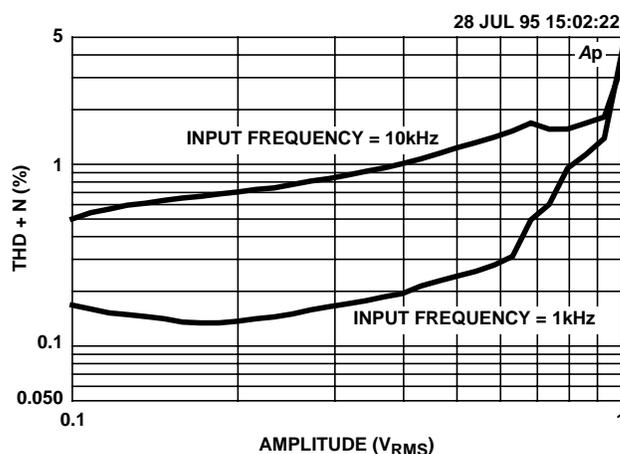
FIGURE 13. THD + N (%) vs AMPLITUDE ( $V_{RMS}$ )
