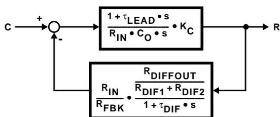
FIGURE 6. COMPLETED CLOSED-LOOP
